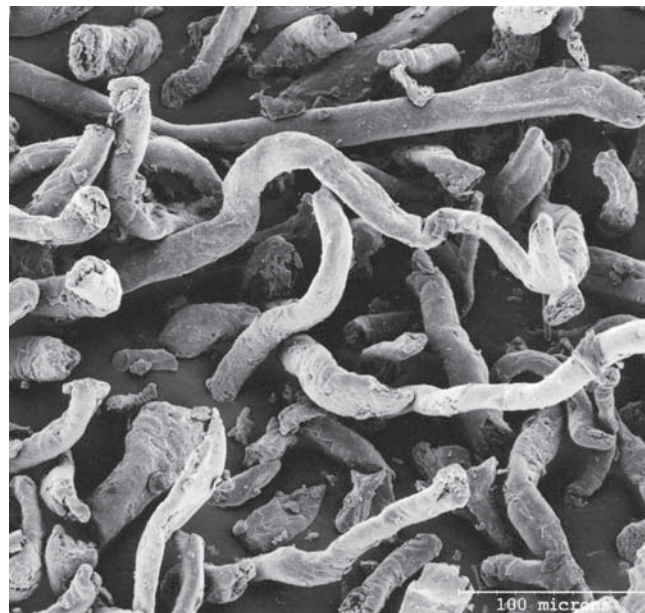
SEM 2: Excipient: croscarmellose sodium ( Ac-Di-Sol ); manufacturer: FMC Biopolymer; magnification: 1000 \times .
