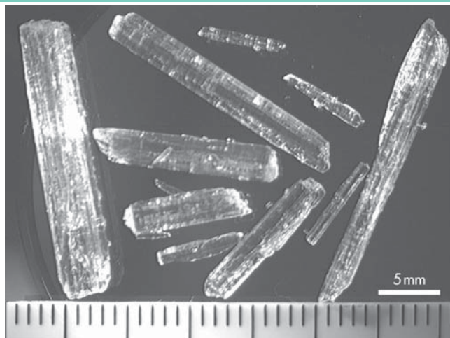
Figure 1: Photomicrograph of large DL-menthol crystals; magnification 7×. Manufacturer: Charkit Chemical Corp., USA.
