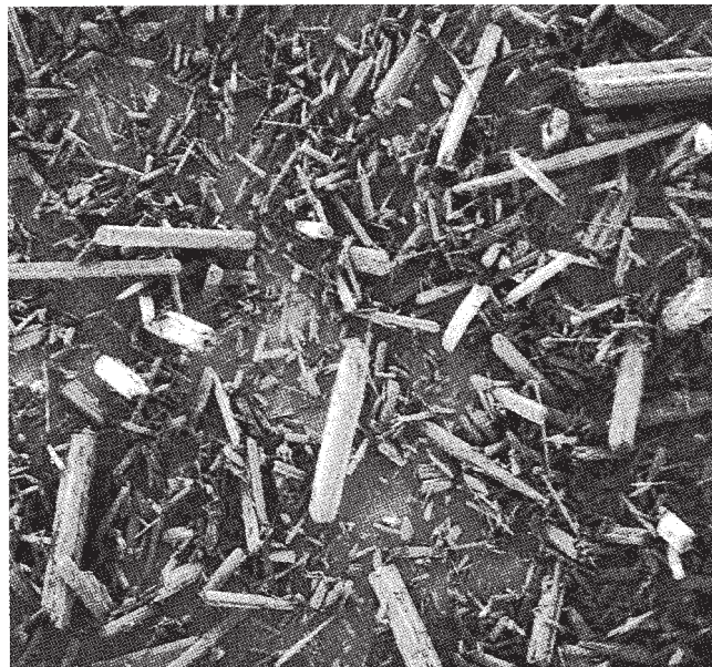
SEM 1: Excipient: aspartame; magnification: 70 \times ; voltage: 3 kV.
